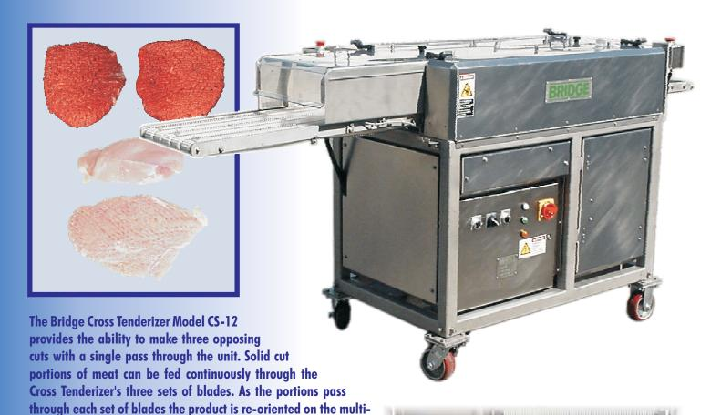
The CS-12 will save you labor and costly production time by eliminating the need for multiple passes through a single unit tenderizer, which would include additional product handling.
