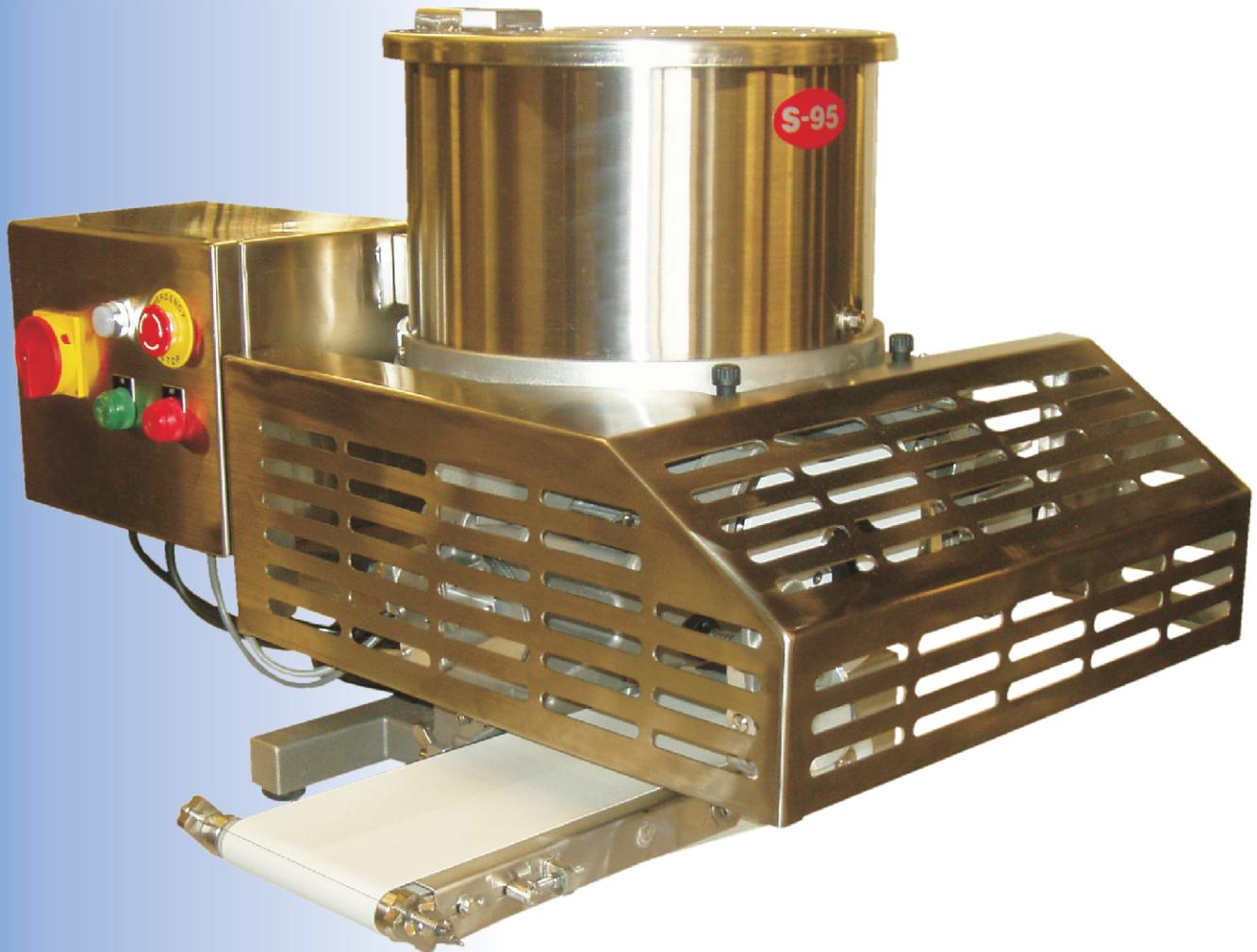
The Bridge Machine S-93 is a drum-type food former designed to form up to 3,200 patties per hour or up to 9,600 meatballs per hour. Form round, oval, square, choppette or natural shape portions with variable thicknesses.
