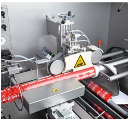
The hot-sealing station of the TSCA provides reliable sealing.
